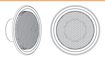
Model PDD-R diffuser provides a displacement system giving improved air quality and lower temperatures in the occupied zone. The diffuser can supply air with very low velocity to avoid draught in the near zone of the diffuser.
